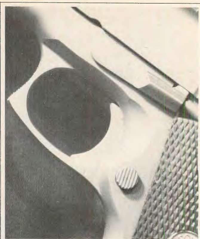
The reshaped trigger guard gives the index finger of the weak hand a solid perch.
